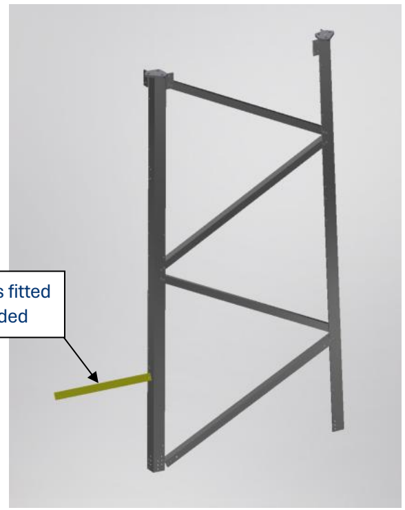
Figure 12. Opposite face with lower diagonal (yellow) fitted to stabilise the face.
