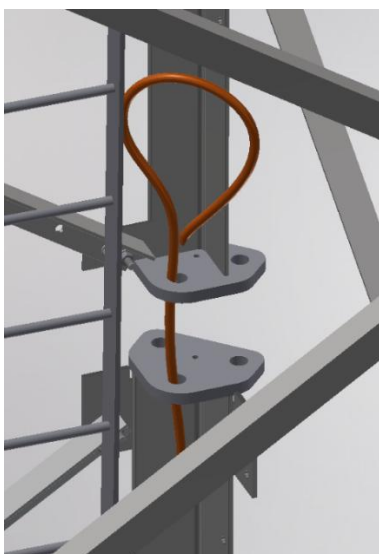
Figure 9. Draw together rope passed through holes to align flanges.
