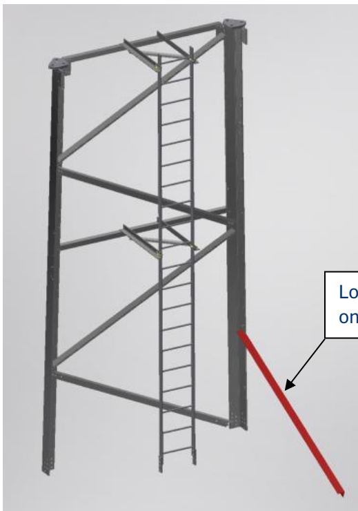
Figure 11. Ladder face with lower diagonal fitted (red) to stabilise the face.
