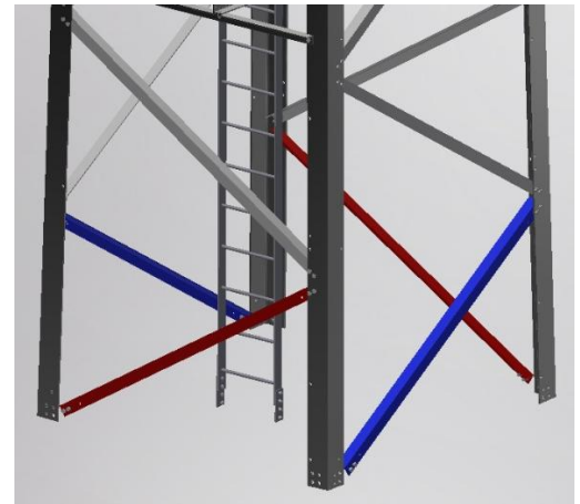
Figure 6. Tower section in vertical position with braces installed in the permanent location ready for landing.
