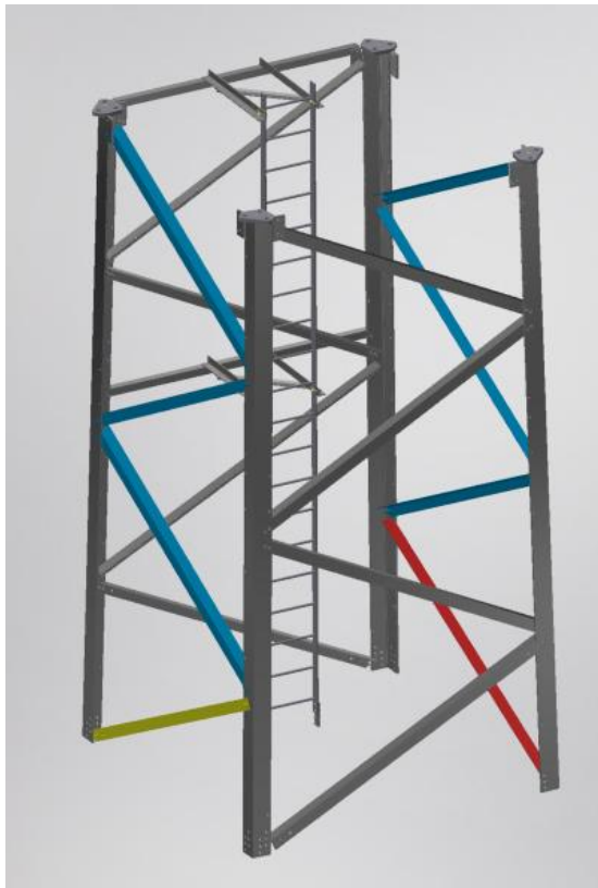
Figure 13. Remaining braces in blue to be hand installed
