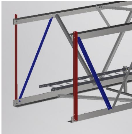
Figure 5. Tower section in horizontal position with braces installed in temporary location for lifting.
