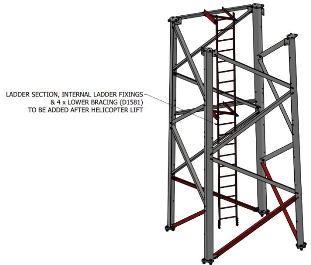
Figure 15. Completed section showing braces and ladder assembly in red to be fitted once module is landed.
