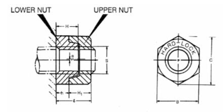
Whilst the tower modules are on the ground, fit the bolt through the parts to be connected and then fit a standard flat washer and the Hard Lock lower nut. It is essential that the lower nut be fitted with the smooth face flush to the washer and fully tightened. Tighten using the 1st stage tightening guidance given above.
