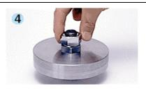
Next, screw the upper (concave) nut onto the bolt by hand.
