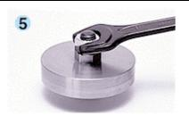
After tightening the upper nut by hand, use a torque wrench to tighten to at least the minimum torque setting given in the Table.
